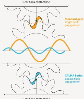
Gear flank contact line
